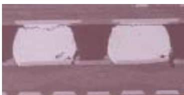
Elemental analysis of solder ball crack areas
